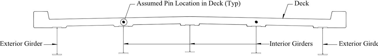
b) Determination of Lateral Distribution of Live Load to Exterior Girders
