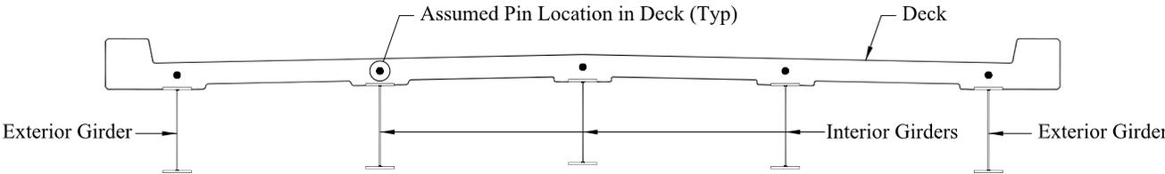
a) Determination of Lateral Distribution of Live Load to Interior Girders
