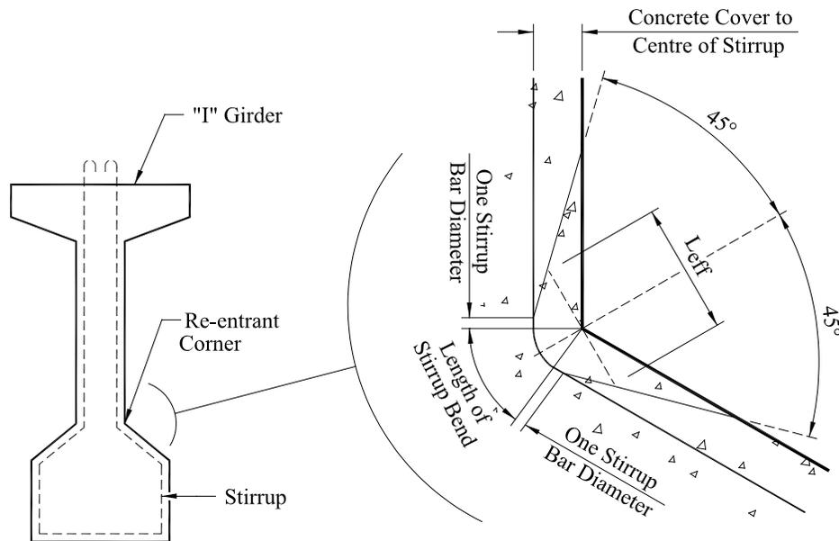
**FIGURE 9.5.5.3 Determination of  $L_{EFF}$  at Stirrup Re-entrant Corner**
