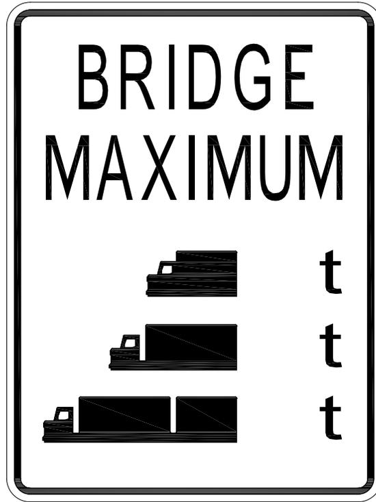
**FIGURE 10** Bridge Load Posting Sign
