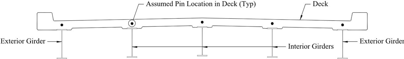
a) Determination of Lateral Distribution of Permanent Load to Interior Girders
