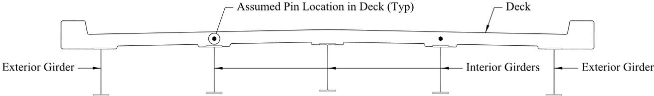
b) Determination of Lateral Distribution of Permanent Load to Exterior Girders
