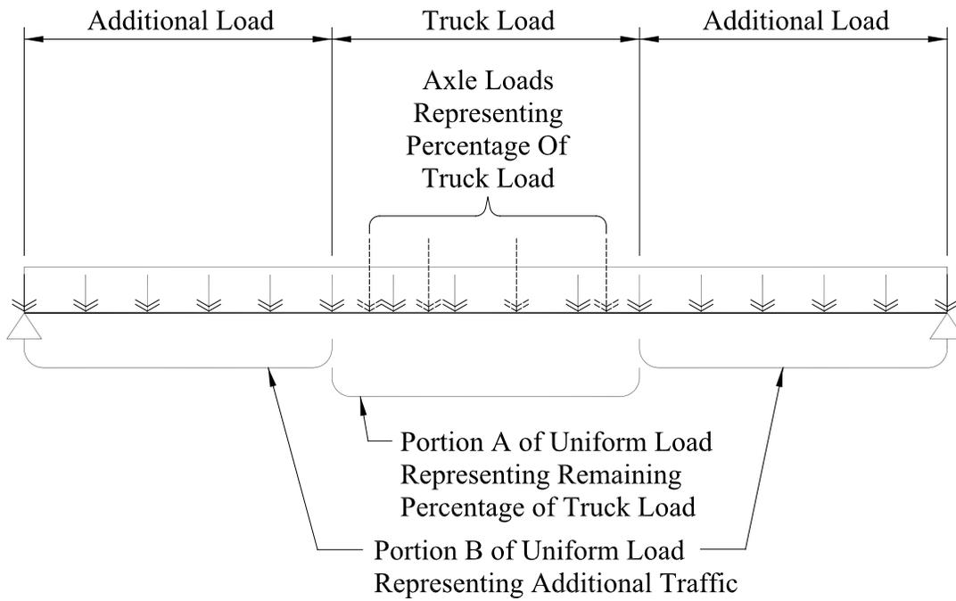
**FIGURE 6.8 Treatment of Uniform Load Portion of Lane Load**
