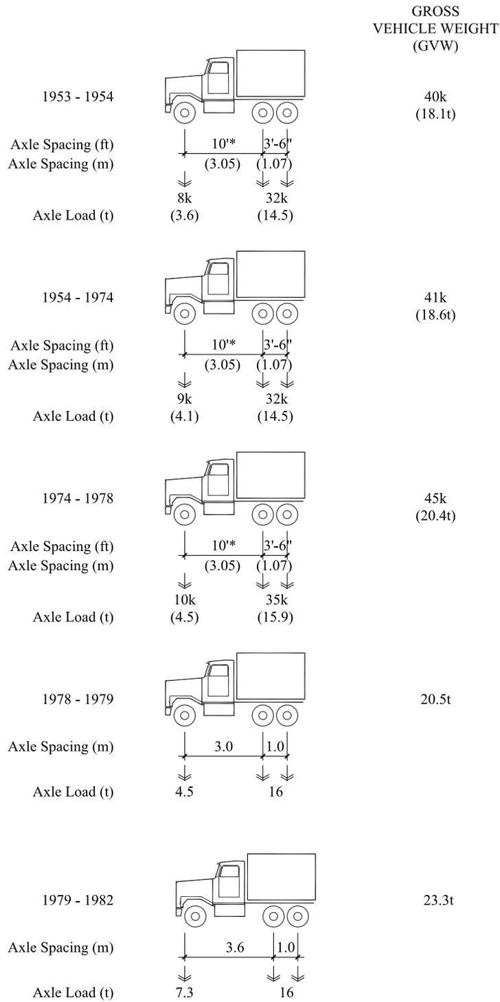
\* Minimum spacing between steering wheel and adjacent drive axle assumed to be 10' (3.05m) although not given in the regulations.
