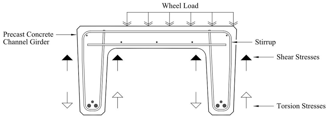
**FIGURE 9.4.4.1 Stirrup Anchorage Requirements in Precast Concrete Channel Girders**
